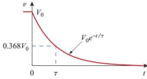
The Time Constant of a circuit is the time required for the response to decay to a factor of 1/e or 36.8 percent of its initial value.
